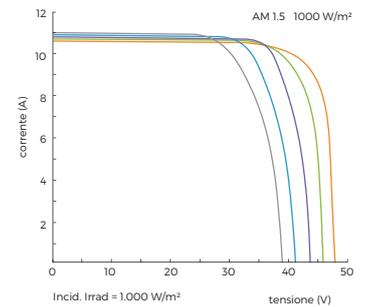
— Oper. Cell Temp. = 0°C — Oper. Cell Temp. = 60°C
